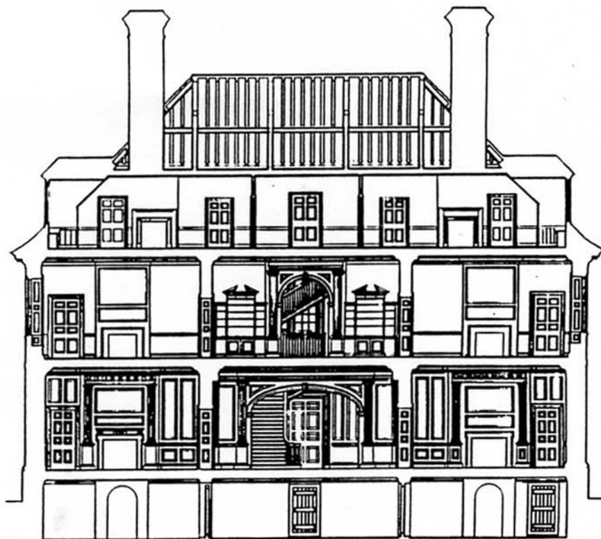
Fig. 1. Section through front rooms, Carter's Grove, James City County. The upper stair, third floor, and roof line date from about 1930. Drawing: E. L. Phillips and J. F. Waite.
